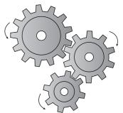
Each cog turns in the opposite direction to the cog it is connected to.
