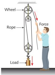
When the rope is pulled down at one end, it lifts the object at the other. With pulleys, it is easier to lift heavy objects, and it is also possible to lift objects higher.
